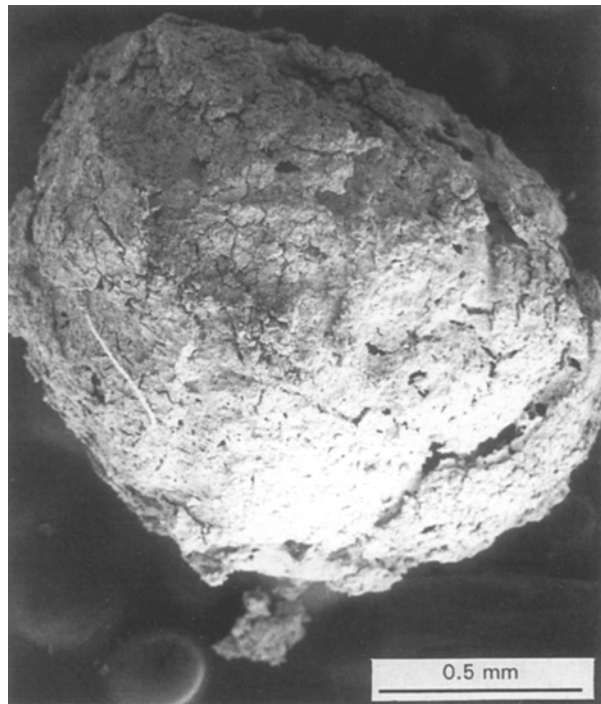
Figure 3 Scanning electron micrograph of a hollow PZT sphere prepared by firing at 850 °C for 4 h.
